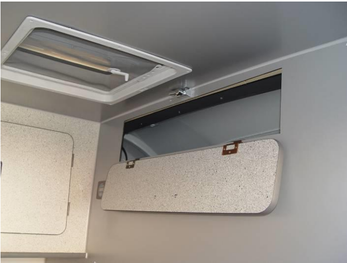
Ventilation lantern and storage space
