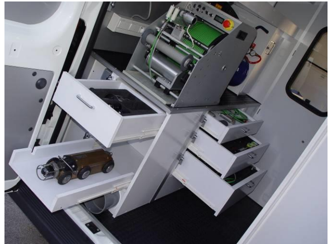
Storage spaces for crawlers and TV cameras
