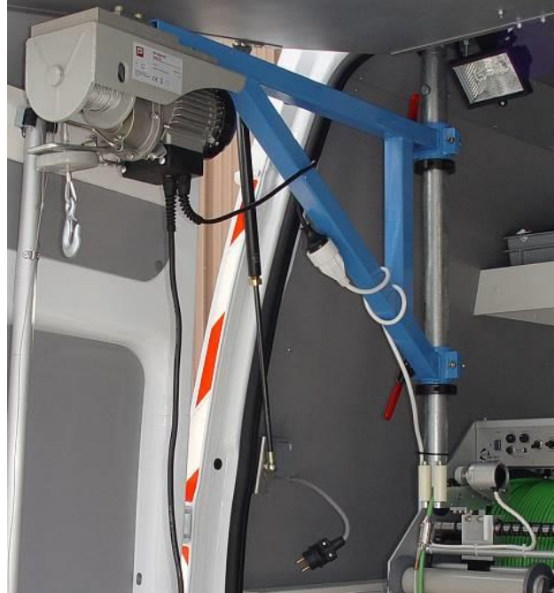
PTSQSP Telescopic jib crane with compact electric winch steel rope 15m
