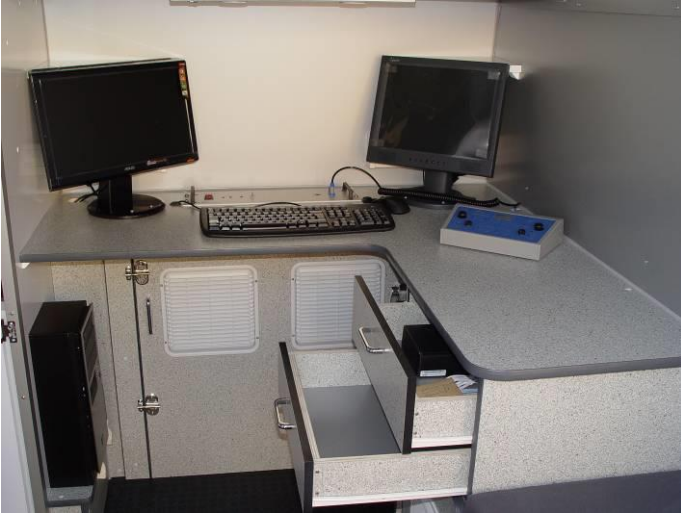
Integration of the VSR65R3U control unit, LCD monitor, digital recorder desktop computer and uninterrupted power supply
