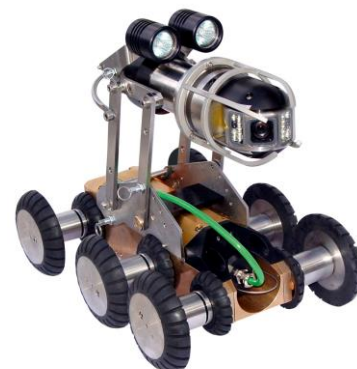
VSCE150X equipped with the FTR80C TV camera for 400 to 600mm diameter configuration
