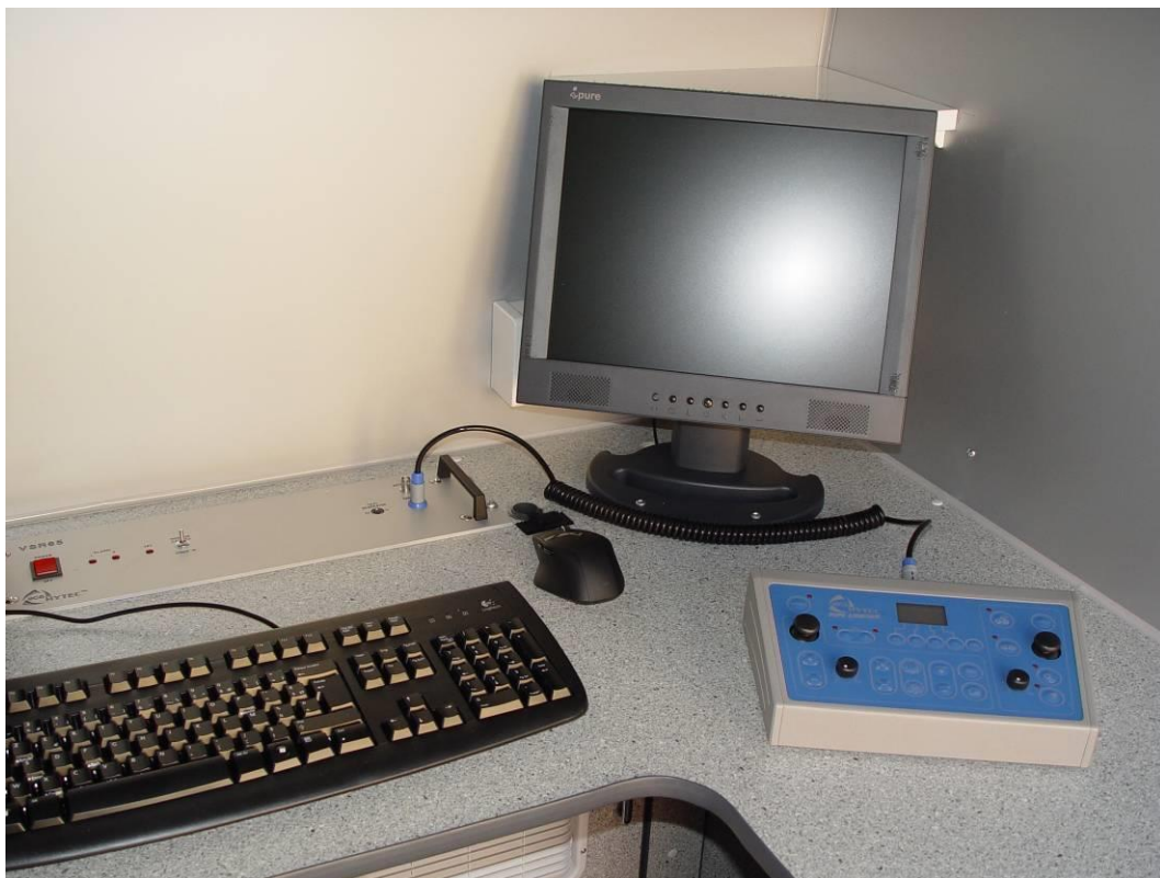
VSR65R3U control unit with its panel control and its 15" LCD monitor
