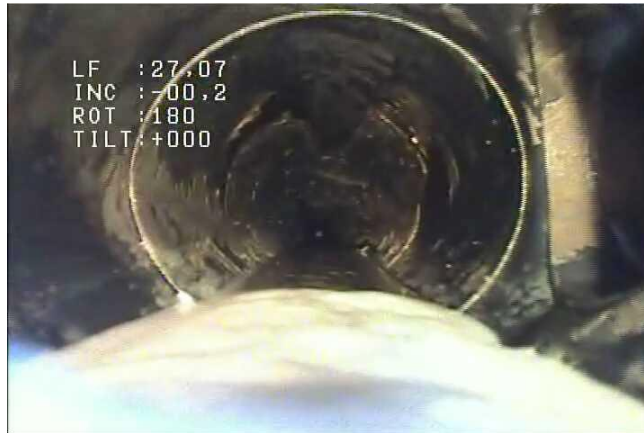
Video picture with camera positions, counting length and inclination data displayed
